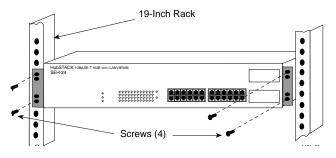
Figure 3-5. Installing the SEH in the Rack
